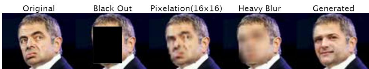
Figure 4.1. Comparison of traditional anonymisation (black-out, pixelation and blurring) versus realistic anonymisation (rightmost image).
