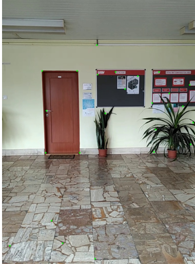
Figure 7: Corner detection with Shi-Tomasi method. Found corners are displayed as green dots.
